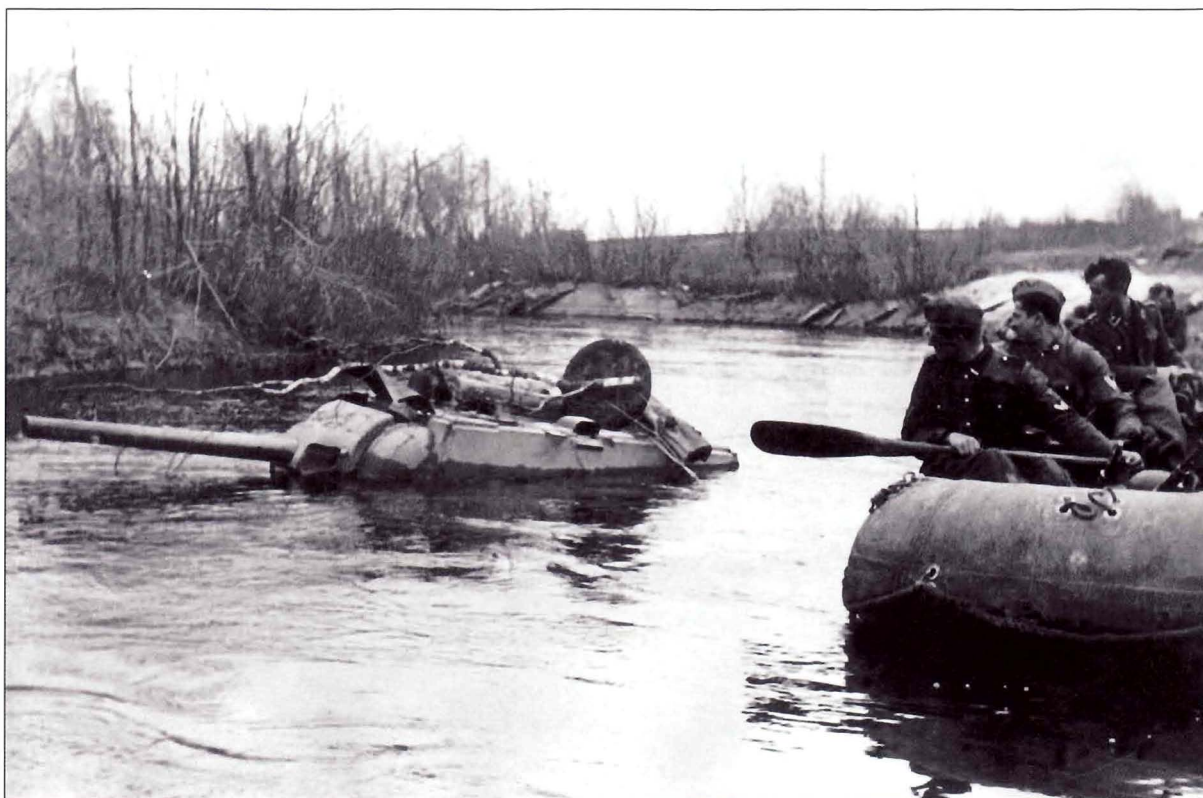
Pioneer troops pause to examine a submerged KV-1 tank as they reconnoiter for a bridge crossing site with the aid of a 5.5-meter (18-foot) medium pneumatic boat. Such boats could carry over a dozen troops. Each boat required a minimum of six paddlers and a steersman. The tank had probably been knocked out or simply mired and abandoned while crossing the stream in summer, when the water was significantly lower.
