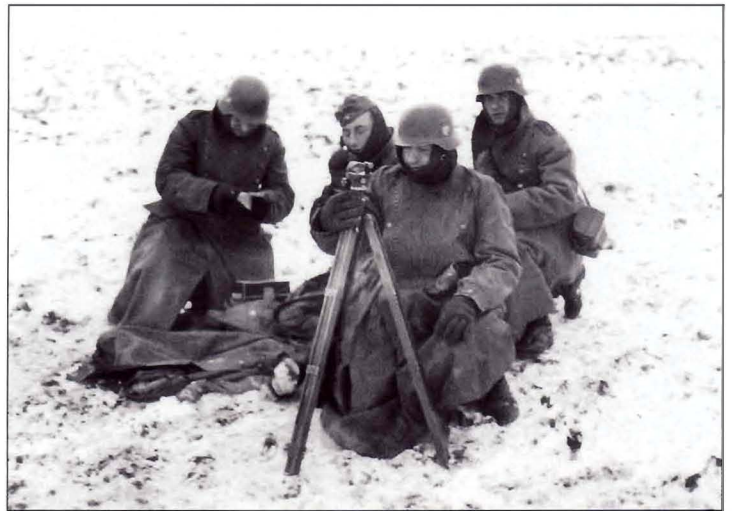
An artillery survey crew operates an Rkr 31 aiming circle (Richtkreis) while setting up an artillery battery. The aiming circle was used to measure vertical and horizontal angles as well as take magnetic bearings like a compass. It was used to setup aiming stakes for each of an artillery battery's four pieces allowing them to be aimed in the same direction even though separated by 30 to 50 meters.
