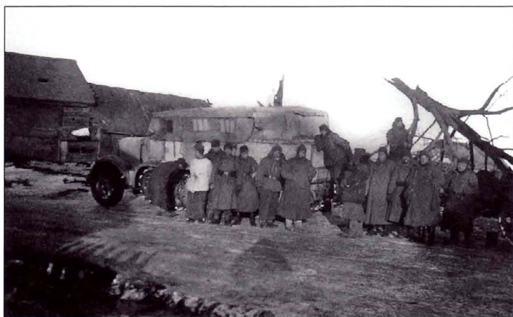
The crew of a 15cm sFH 18 heavy field howitzer pose beside their 12-ton SdKfz 8 heavy halftrack (schwerer Zugkraftwagen). The latter was the standard prime mover for 15cm howitzers and guns, 10cm guns, 21cm mortars, and 8.8cm and 10.5cm Flak pieces. The halftrack is seldom seen with the canvas weather top erected.
