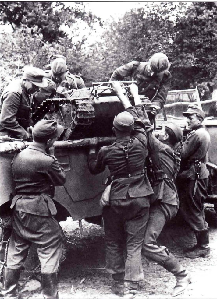
Pioneer troops struggle to unload a 370-kilogram (816-pound) SdKfz 303a "Goliath" light demolition carrier (leichter Ladungsträger) from a field car. This gasoline-driven vehicle was remotely controlled via a 650-meter (2,133-foot) wire and carried a 75-kilogram (165-pound) TNT charge. The longer SdKfz 303b version carried a 100-kilogram (220-pound) charge. A smaller and earlier version, the SdKfz 302, driven by an electric motor and carrying a 50-kilogram (110-pound) charge had seen use. A number of "Goliaths" were captured at Normandy where they proved to be ineffective for attacking beached landing craft. This gave them a bad reputation. On other fronts they were effectively employed against fortifications, defended buildings, and major obstacles, especially antitank barriers and walls.
