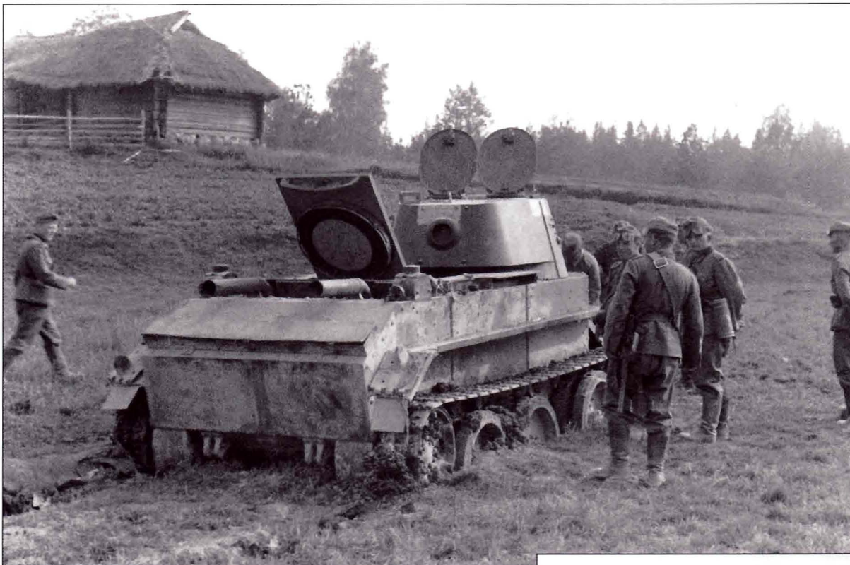
Troops examine an abandoned Soviet BT-7 light tank that had become bogged down in a muddy field. Almost as many tanks were lost to this cause as by gunfire buy both sides. Of course many of the mired tanks were shot up anyway after they were abandoned. This one, armed with a 45mm gun, appears to have been spared and might eventually see German service for rear area security.
