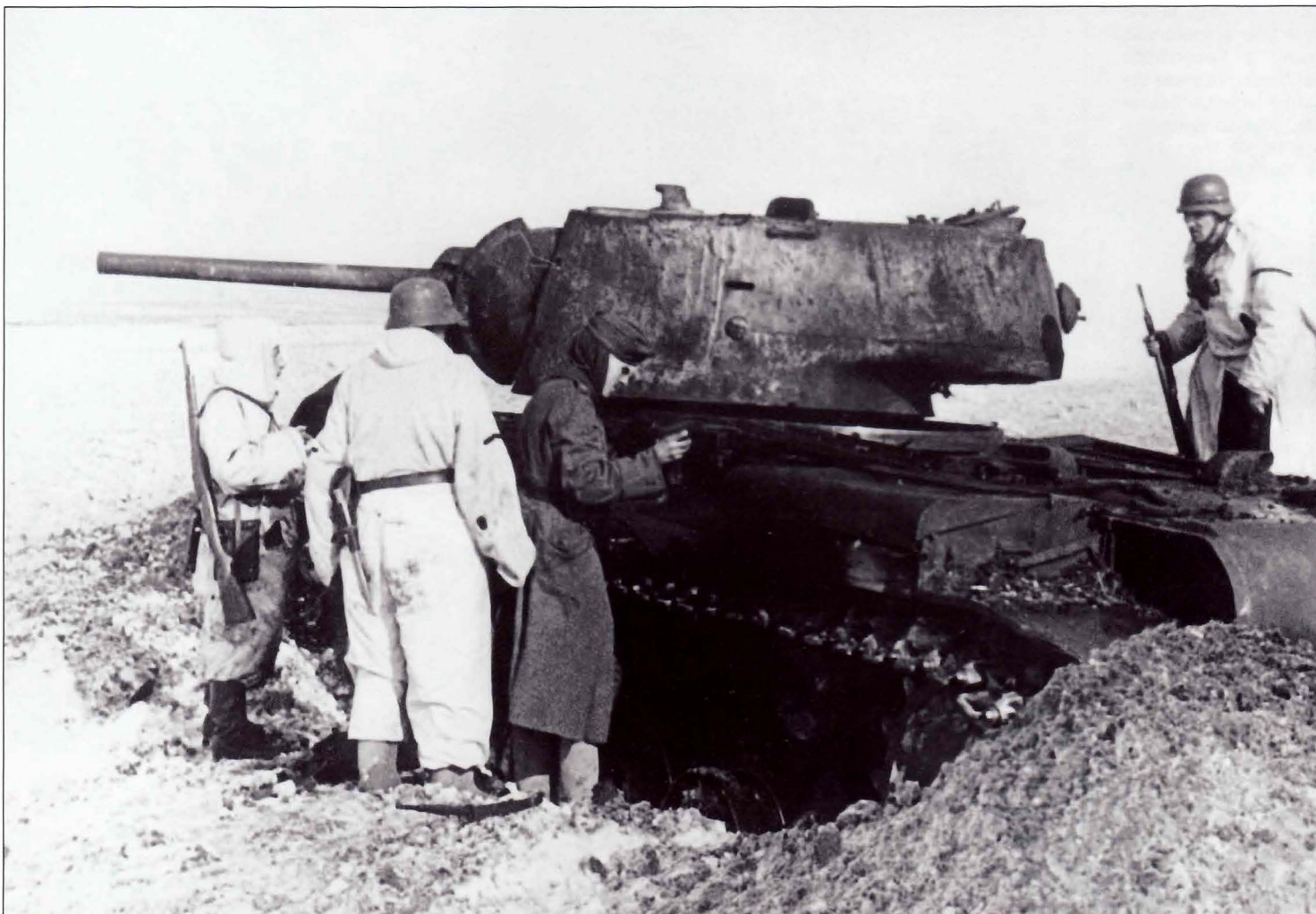
This scorched KV-1 has been partly dug-in, but this effort did not protect it. The small "doom" on the rear of the turret is a mounting for a 7.62mm DT machine gun.
