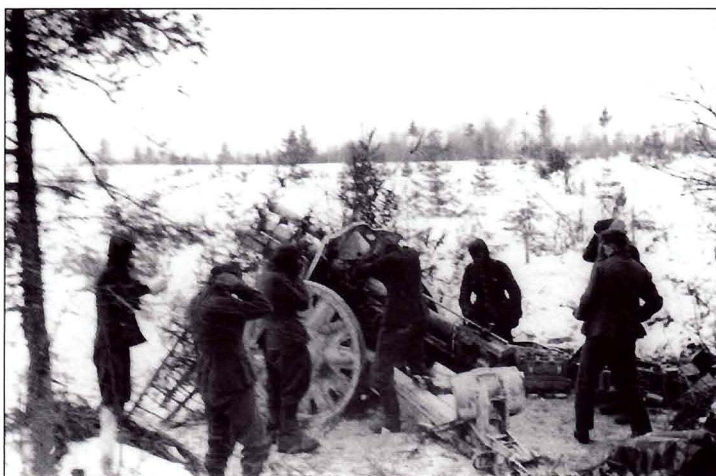
A 10.5cm leFH18 light field howitzer in full recoil. The crew is wearing only the standard wool field uniform without any protective clothing other than some wearing gloves and some form of over boots. Note the litter of wicker baskets, boxes, and cans for projectiles, propellant cartridges, and fuses scattered around the gun. The gun appears to have been whitewashed.
