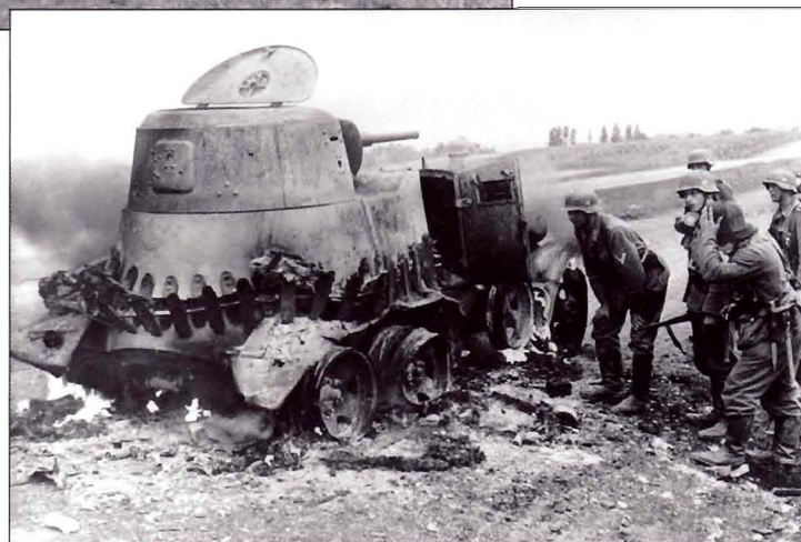
This completely burned out Soviet BA-3 armored car is being examined by infantrymen. The BA-3 was armed with a 45mm gun and 7.62mm DT coaxial machine gun in the turret of a T-26 tank. It was built on a GAZ-AAA truck chassis. There was no power to the front wheels. To improve mobility on soft ground comparatively lightweight tracks could be fitted to the two pairs of rear tires. These are seen stowed on the rear hull.
