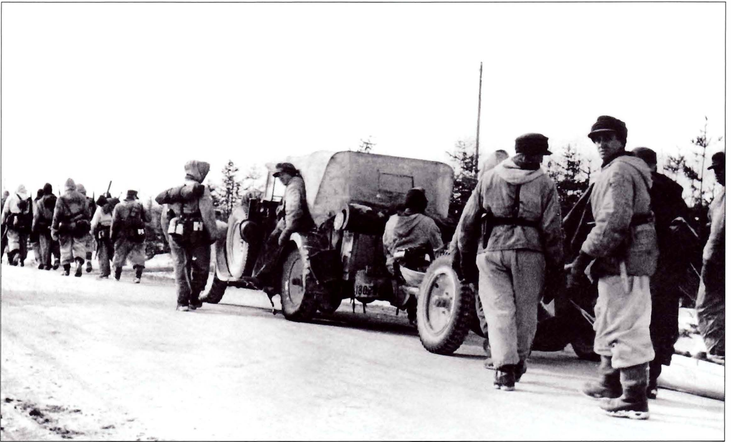
Wearing reversible winter uniforms, troops move toward the front. A Kfz 11 medium cross-country personnel car tows a 3.7cm Pak 35/36 antitank gun. Note that the car's and gun's wheels are the same, making them interchangeable. Antitank guns were provided motorized prime movers if at all possible to allow them to be moved into position rapidly and repositioned quickly. This maximized their survivability and ability to meet new threats.
