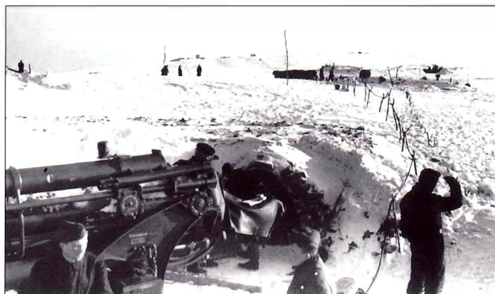
The crew of a Luftwaffe 8.8cm Flak cleans up the gun emplacement. Note the cable suspended on Y-shaped poles that connects the gun fuse-setter to the fire director located in the center of the four-gun battery position.
