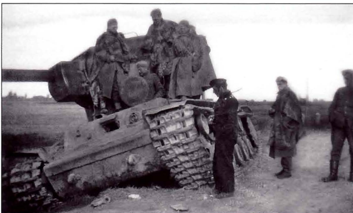
Along with other troops a Panzer Unteroffizier examines a KV-2 heavy tank or "artillery tank." No doubt he is practically interested in this formidable monster. Though its 110mm armor made it difficult to kill, the exceedingly high turret made an excellent target. Most were lost early in the invasion. This turret was mounted on a KV-1 chassis. The 334 KV-2s were intended as infantry support assault guns for destroying bunkers and were usually armed with a 152mm gun, though some had a 122mm. A few were employed by the Germans.
