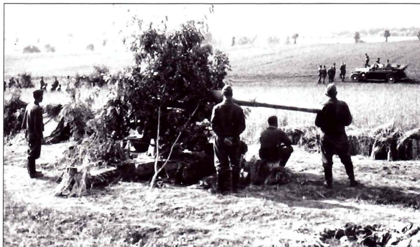
Luftwaffe 8.8cm Flak 18 crew watches as staff officers discuss unit dispositions. The gun is well camouflaged and the limbs can be quickly pulled away when an air alert is given. Even the gun mount is camouflaged with straw as are the ammunition crates to the right and the crew tent shelters to the left.
