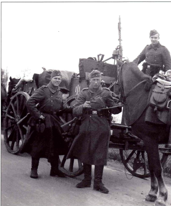
This artillery unit (signified by the white artillery tactical symbol) has mounted an MG34 machine gun on a caisson for antiaircraft protection. This may be the two-caisson-type communications wagon provided to artillery batteries. Artillery caissons and gun limbers had over-the-wheel fenders, which these wagons lack. Note the brown leather M1934 saddle bag on the horse to the right.
